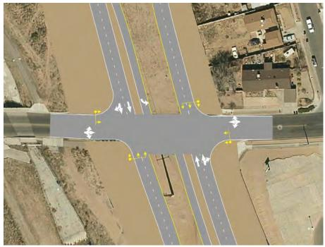
Figure 16 - Single Point Intersection Signalization
