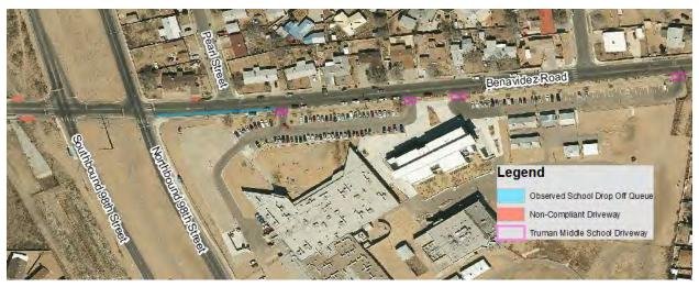
Figure 4 - Driveways Based on Proximity to the Intersection
