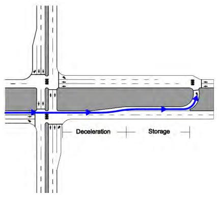
Figure 20 - Placement of Median U-turn
