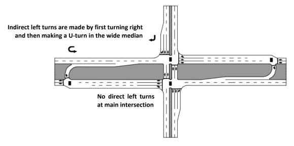
Figure 18 - Indirect Left Typical Lane Configuration
