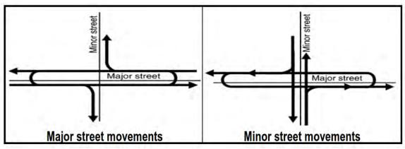
Figure 17 - Vehicle Movements through Indirect Left Treatment
